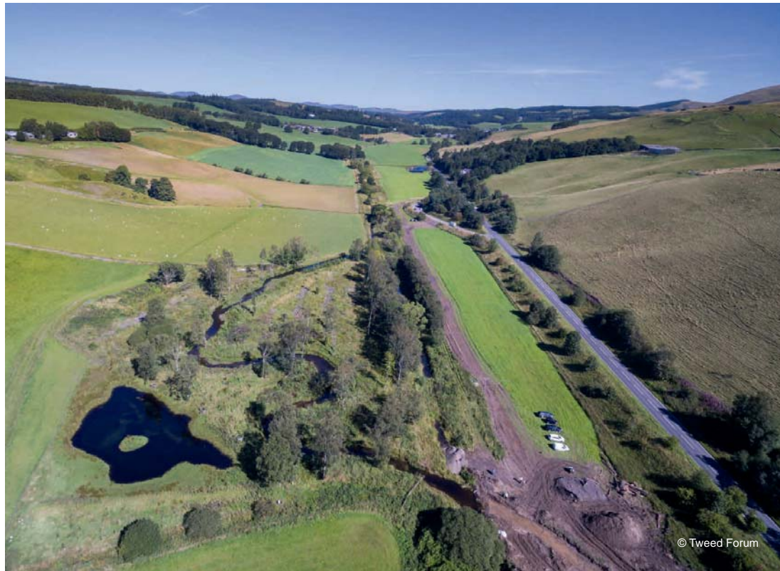
River landscape restoration in the Eddleston Water catchment of the river Tweed has included the re-meandering of 3km of straightened watercourses.
